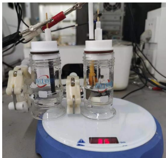
Figure S2. Reaction setup for the electrochemical synthesis of amino acids over a Ni NF cathode.
