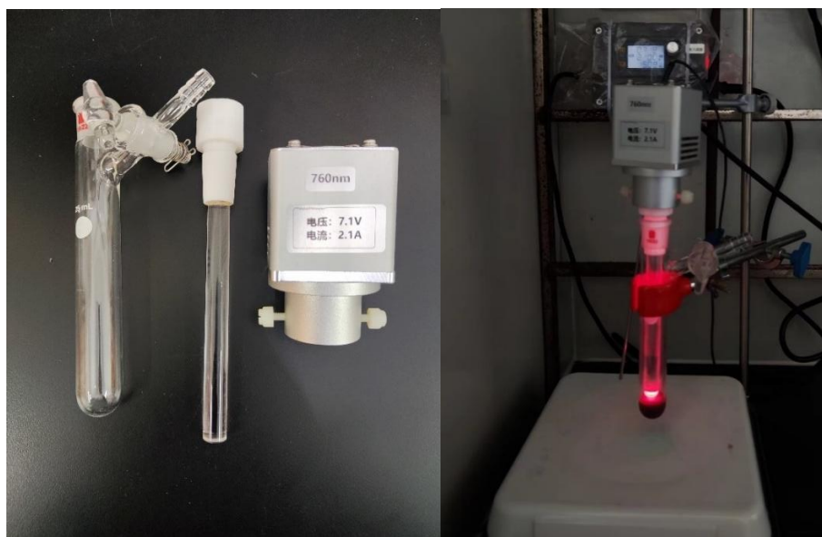
Figure S9. Photoreactor setup used in this study.
