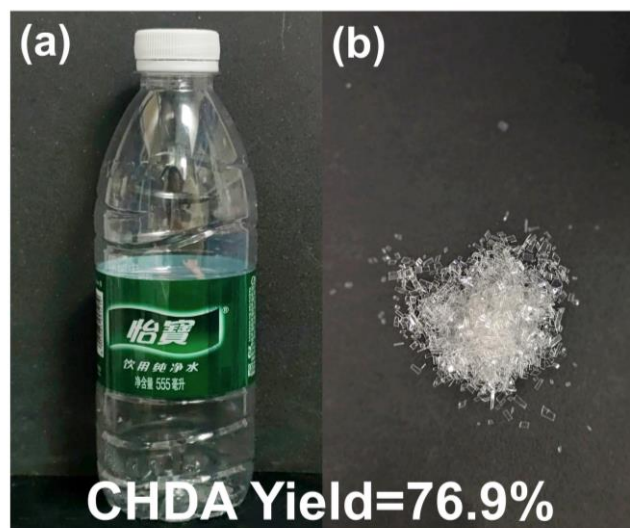
Figure S8 Photograph of (a) PET bottle and (b) the fragments of the PET bottle after processing.
