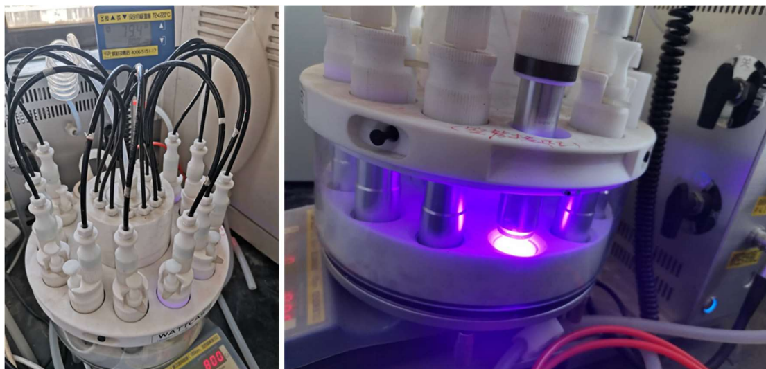
Figure S4. Pictures of the photocatalytic parallel reaction apparatus
