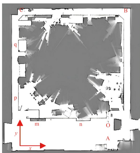
图9 EAST大厅二维栅格地图 Fig.9 2D grid map of the EAST hall
