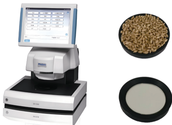
图1 本试验中使用的近红外检测仪 DA7250 和小样品盘 Fig. 1 Near-infrared reflectance spectrometer DA7250 and small sample tray used in this experiment
