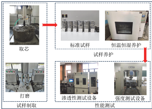
图8 试样制作和试验设备 Fig.8 Sample preparation and test equipment
