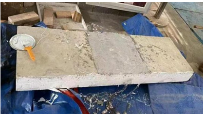
图 3 下贴纤维复材的试件板底 Fig. 3 Schematic diagram of the bottom of the slab with fiber composite material
