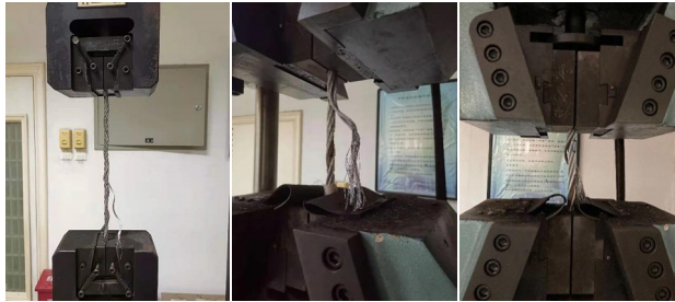
图 22 钢丝绳试样破坏状态 Fig. 22 Failure states of steel wire rope samples
