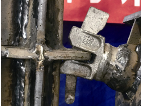
图 7 横杆抗弯试验破坏形式 Fig.7 The failure modes of the transverse tube in bending test
