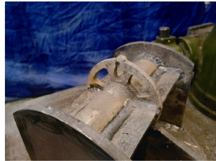
图 10 横杆抗拉试验破坏形式 Fig.10 The punch failure mode of the transverse tube in tensile test
