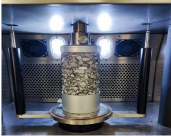
图7 四种混合料蠕变变形量试验过程 Fig.7 Test process for creep deformation of four asphalt mixtures
