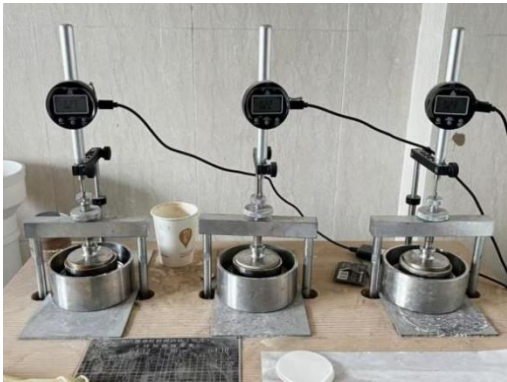
图6 三联杠杆式压缩固结仪 Fig.6 Three-lever compression consolidation apparatus
