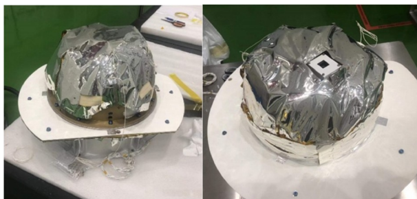
图3 (网络版彩图)穹顶舱外部热控实施 Figure 3 (Color online) Implementation of external thermal control in the dome cabin.
