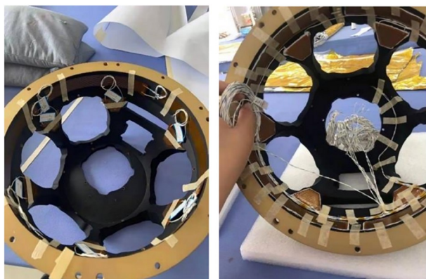
图2 (网络版彩图)穹顶舱内部热控实施 Figure 2 (Color online) Implementation of internal thermal control in the dome cabin.
