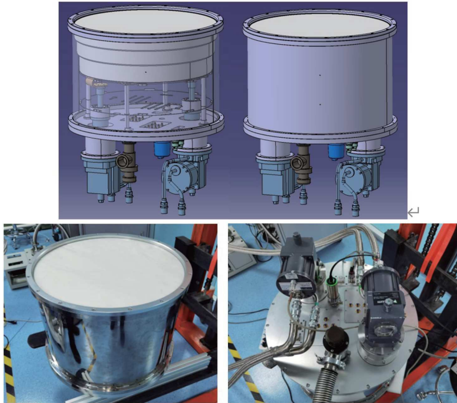
图 3 平面型真空窗低温杜瓦 Figure 3 Planar vacuum window cryogenic dewar.
