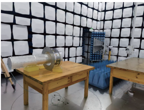
Fig. 7. The combined OMT and feed, and the E-plane far-field directional pattern of the feed in the 1.42 GHz, in the microwave anechoic chamber at the FAST project site.
